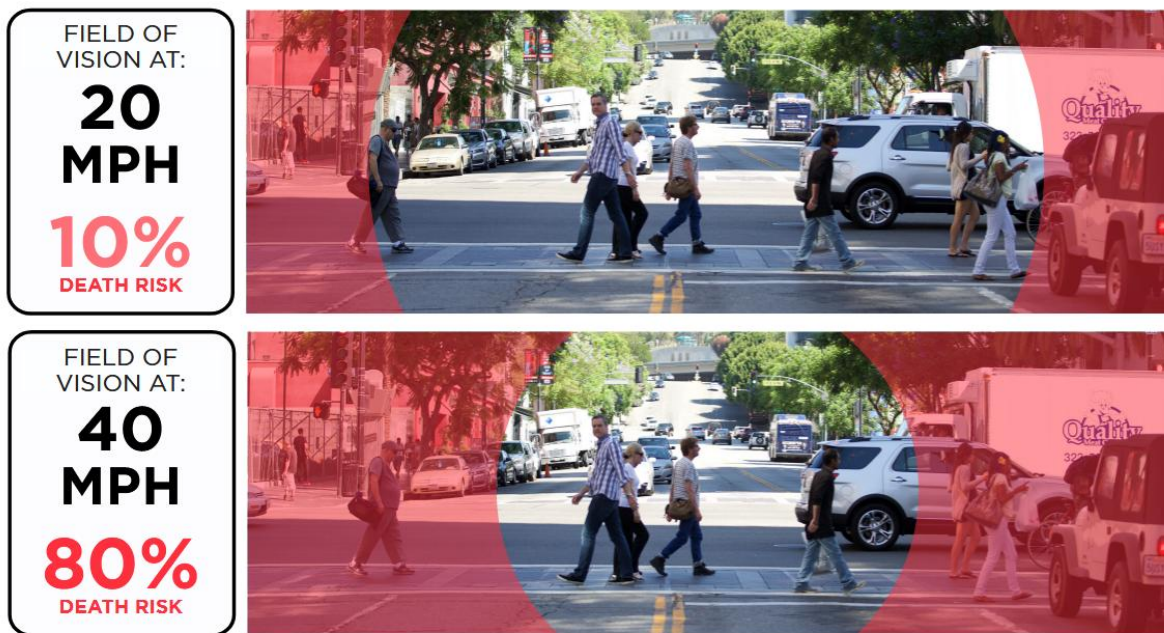
The effect of vehicle speed on a driver's field of vision and the chance of pedestrian death in a crash. Image: LADOT.
