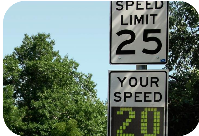
A vehicle-activated feedback sign. Photo credit: Richard Drdul/Wikimedia Commons.
