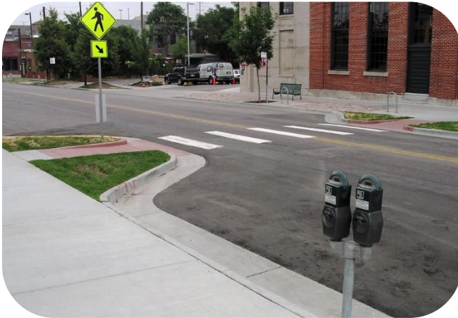
Mid-block curb extensions or "bulb-outs" to reduce vehicular speed and pedestrian crossing distance. Photo credit: Richard Drdul/Wikimedia Commons.
